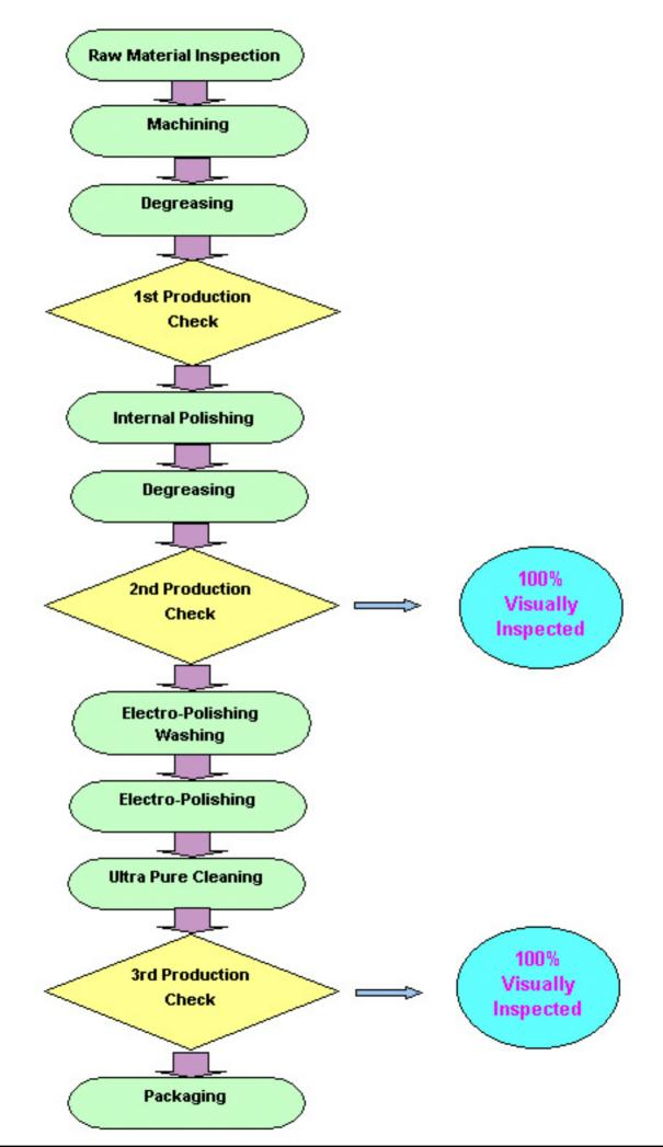
After CNC machining, cleaning and electropolishing, all components are ultrasonic cleaned, rinsed a boiled with 18 Megohm D.I water, and blow dried at 250°F and purged with filtered hot N<sub>2</sub> gas prior to packaging.
